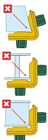
WARNING CORNERMAX® PAD CUT PROTECTION Damaged or misused protection can result in damage or sling failure. Inspect before each use. Inspect for cuts, tears or damage that may prevent protection of the sling. Ensure protection is the correct size and type to protect the sling. Prevent pads and sling from slipping or sliding across load edge. DEATH or INJURY can occur from improper use, maintenance and/or inspection. MAXIMUM LOADING: Do NOT exceed 25,000 lbs. per inch of sling width.
